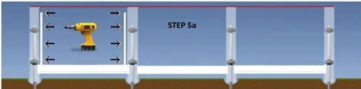
**STEP 5a: Fastening on U-Channels.** Screw U-Channel to vinyl posts using (4) #10 x 1" screws.
